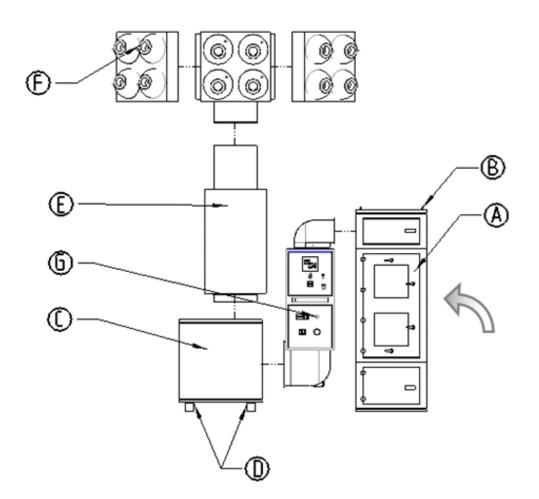
• First the filter component (A) as delivered must be transported to its destination. There the filter component (A) must be moved to an upright position. Therefore, lift the filter component (A) with lifting tools by using the lifting rings (B).
